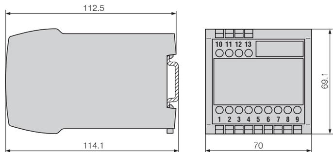
Fig. 4. SINEAX B 840 in housing **P13/70** clipped onto a top-hat rail (35 × 15 mm or 35 × 7.5 mm, acc. to EN 50 022).
