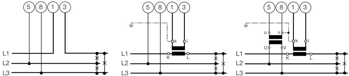
Connect the voltage according to the following table for current measurement in L2 or L3:
