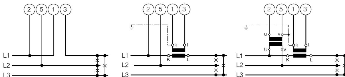
Connect the voltage according to the following table for current measurement in L2 or L3:
