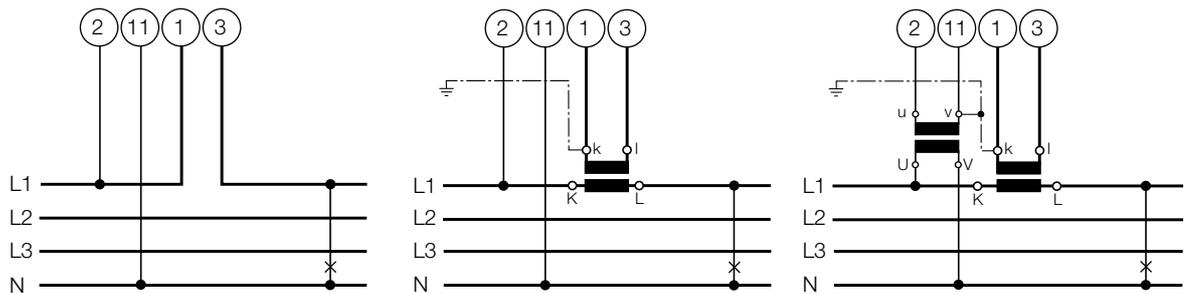
Connect the voltage according to the following table for current measurement in L2 or L3:
