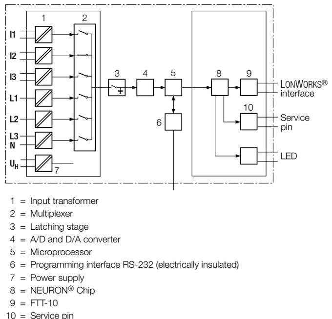
Fig. 2. Block diagram.
