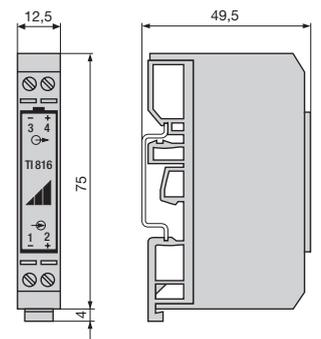
Fig. 10. SINEAX TI 816 on top-hat rail EN 50 022 – 35 × 7.5.
