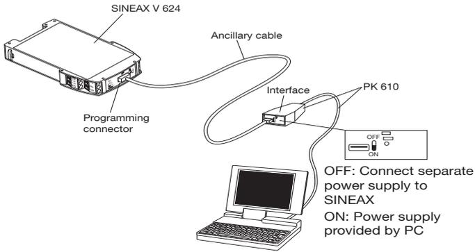
Fig. 6. Configuring a SINEAX V 624 without the power supply. For this case the switch on the interface must be set to "ON".
