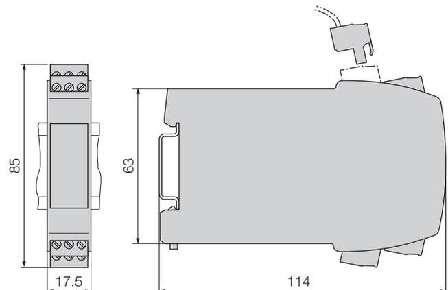
Fig. 12. SINEAX V 624 in housing **P12/17 St** clipped onto a rail «G» (35 × 15 mm or 35 × 7.5 mm, acc. to EN 50 022), **screw terminals pluggable**.
